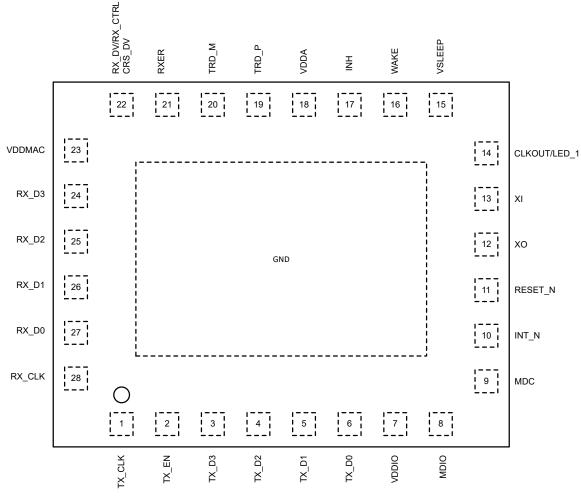
Figure 4-2. DP83TC813R-Q1 Pin Diagram
