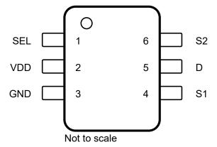
Figure 4-1. Pin Diagram (SOT-23 Package)
