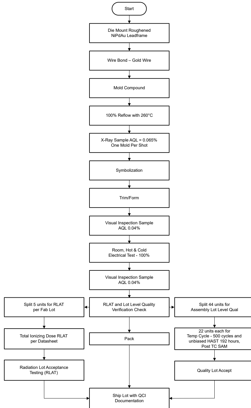
Figure 1-1. TXGS441-SEP Space Enhanced Plastic Production Flow Chart
