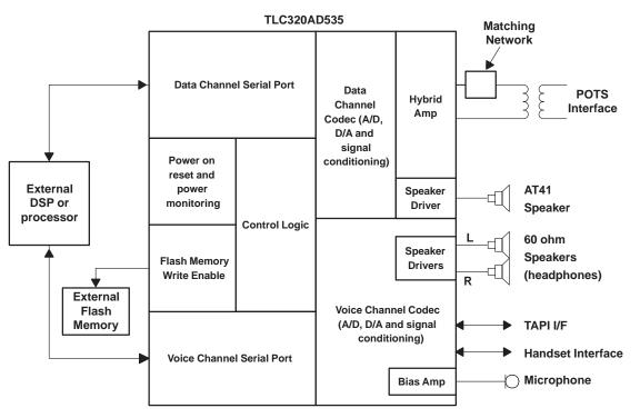
Figure 2. TLC320AD535 Block Diagram
