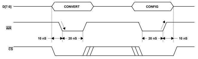
Figure 2. ADS8364 Write Timing
