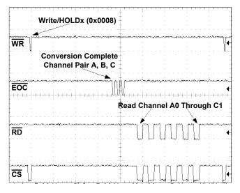
Figure 3. ADS8364 Waveforms
