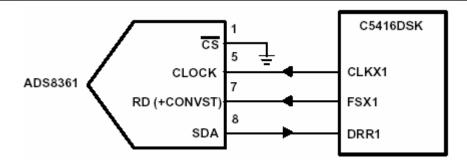
Figure 1. Hardware Interface Block Diagram
