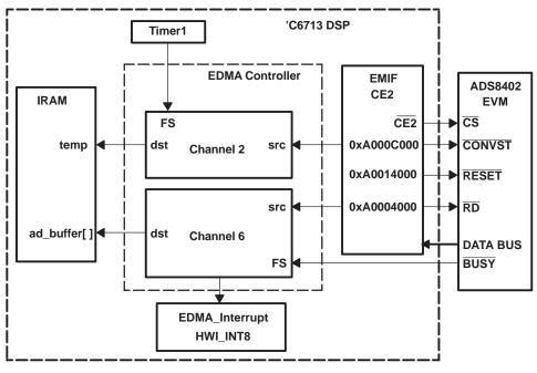
Figure 2. Data Transfer Block Diagram Using EDMA
