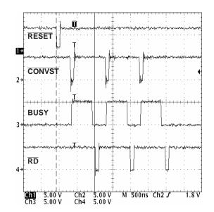
Figure 4. Scope Screenshot Showing Power-On Initialization Cycles
