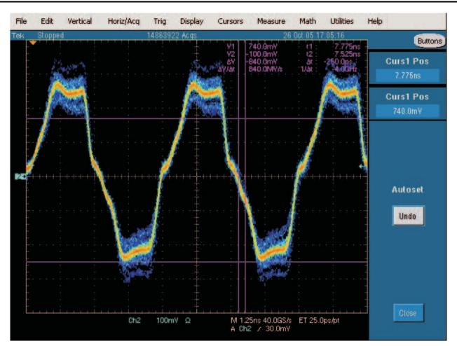
Figure 9. CLK\_O at the Receiver End Using Cable
