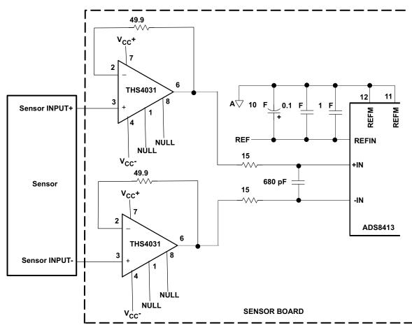
Figure 5. Sensor and the ADC (Analog Side)
