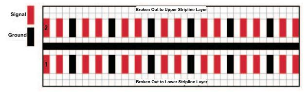
Figure 2. Connection to Make 100- $\Omega$  Differential Impedance Matching
