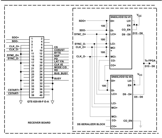
Figure 7. LVDS to 16-Bit Parallel De-Serialization
