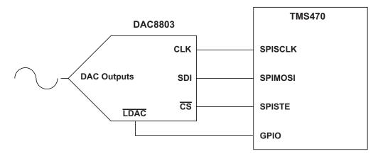
Figure 1. Basic Hardware Interface
