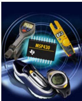
Take full advantage of the capabilities of TI's MSP430. Add a 32.768 kHz crystal to your MSP430 controller and you'll generate an accurate reference frequency for the microcontroller's sleep mode, as well as your other circuitry that may require a timing reference.
