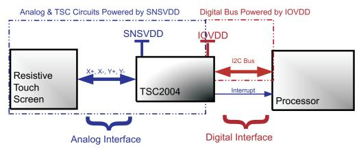
NOTE: Note that the supply voltage on IOVDD must be the same as or lower than SNSVDD
