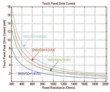
The touch screen is driven by touch screen controller; the panel's resistance determines the peak drive current from the touch screen controller from the SNSVDD power supply.
