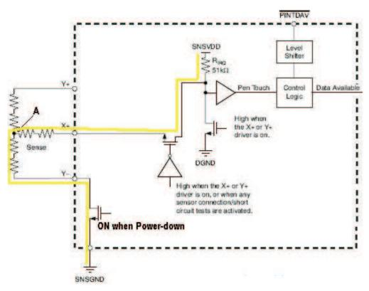
Figure 2. TSC Internal PENIRQ Circuit
