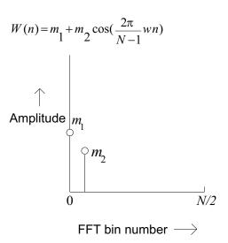
Figure 7. Spectrum of Window Function
