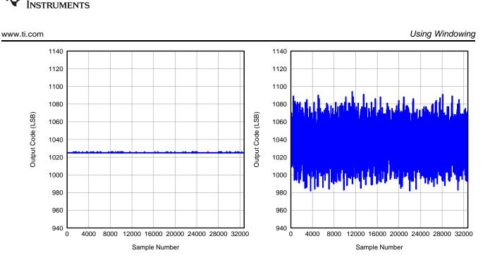
Figure 3. Time Domain Data With SNRBoost<sup>36</sup> Disabled and Enabled (With No Input Signal)
