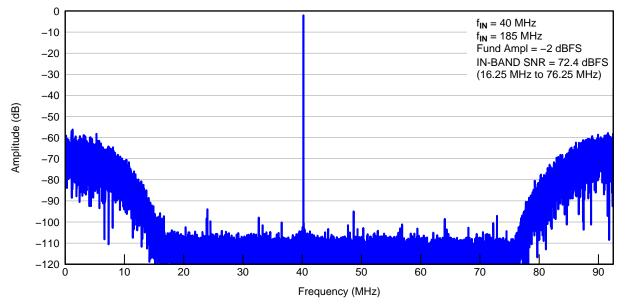
Figure 1. Spectrum of Signal With SNRBoost<sup>3G</sup> On
