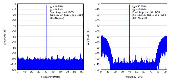
Figure 2. Full-Band SNR Comparison With SNRBoost<sup>3G</sup> Disabled and Enabled
