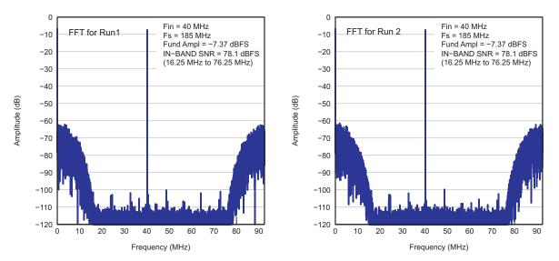
Figure 5. Stable Spectrum With SNRBoost<sup>36</sup> Enabled and After Windowing
