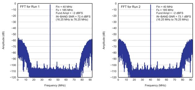
Figure 4. Unstable Spectrum With SNRBoost<sup>3G</sup> Enabled
