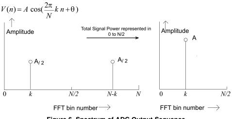
Figure 6. Spectrum of ADC Output Sequence
