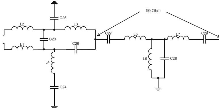
**Figure 2. 50- $\Omega$  Points in the Balun**
