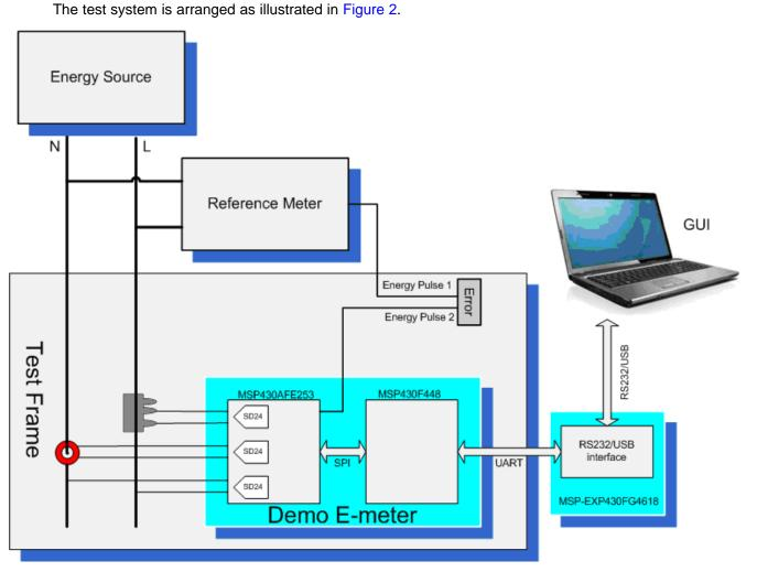
Figure 2. Test System Setup
