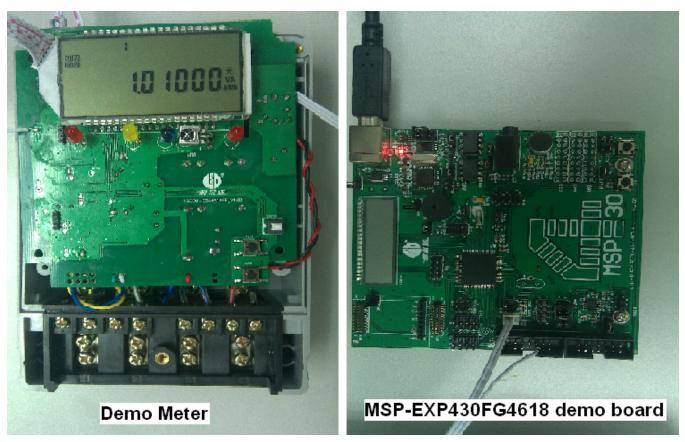
Figure 1. Demo Meter and MSP-EXP430FG4618 Demo Board
