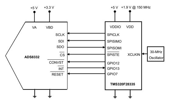
Figure 1. Hardware Connection
