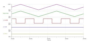
Figure 5. Fault Indication Waveform
