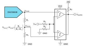
Figure 6. Resource Optimized Fault Indication
