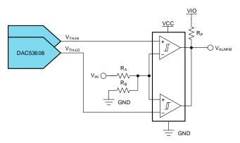
Figure 4. Window Comparator for Fault Indication
