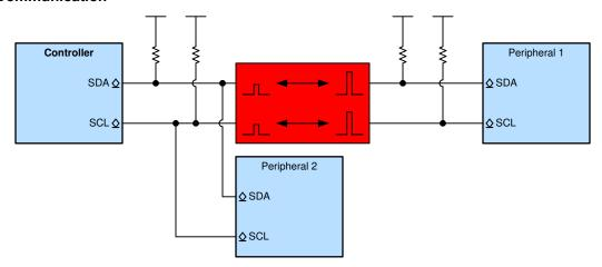
Figure 2-10. Using Voltage Translation with an I<sup>2</sup> Communication Bus
