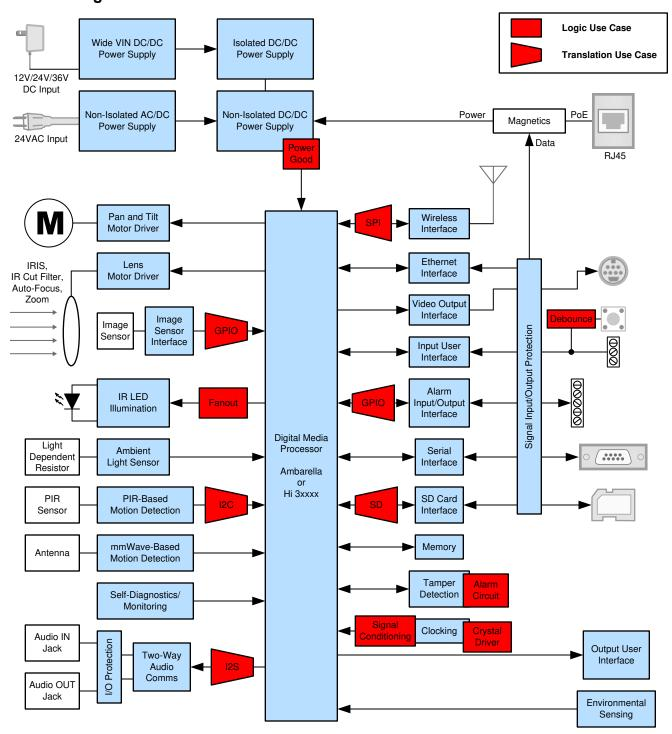
Figure 1-1. Simplified Block Diagram for IP Cameras
