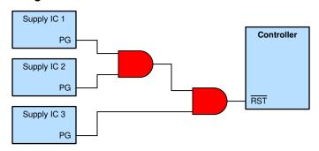
Figure 2-1. Using Logic to Combine Multiple Power-Good Signals
