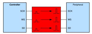
Figure 2-12. Using Voltage Translation with an I2S Communication Bus
