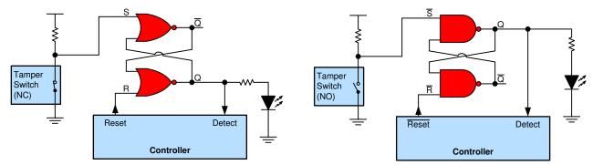
Figure 2-4. Using Logic to Monitor a Normally Closed (NC) Tamper Switch
