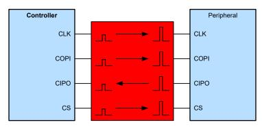
Figure 2-8. Using Voltage Translation with a SPI-communication Bus
