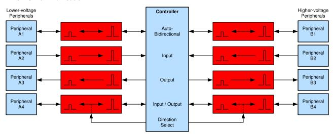
Figure 2-9. Using Voltage Translation with GPIO Communications
