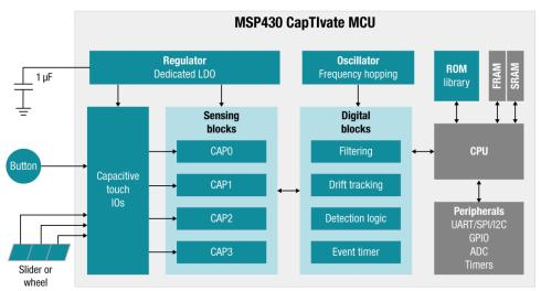
Figure 2-1. MSP430 Capacitive Sensing MCU Block Diagram
