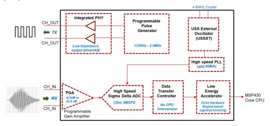
Figure 1-1. TI's Ultrasonic Subsystem
