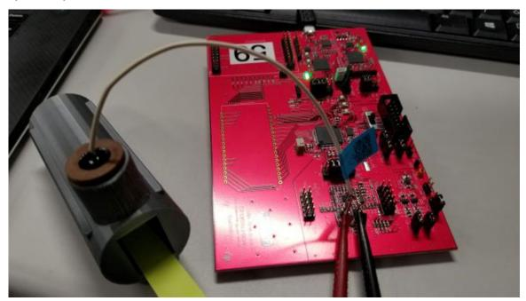
Figure 2-1. 3D Printed Fixture and EVM
