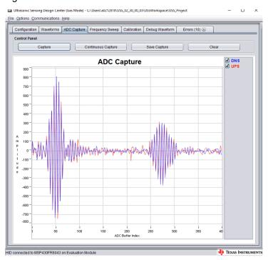
Figure 2-3. First and Second Ultrasonic Reflections
