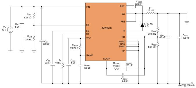
• RT sets the oscillator switching frequency. Generally, higher-frequency applications are smaller but have higher losses. Operation at 500 kHz was selected for this example as a reasonable compromise for both small size and high efficiency. RT is calculated using the following equation:
