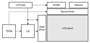
Figure 1-1. Typical LCD Panel Subsystem Diagram Block
