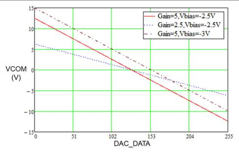
Figure 1-3. LCD Digital VCOM Voltage Characteristic
