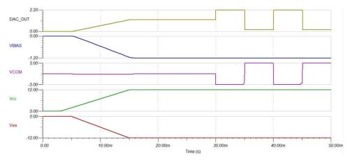
Figure 3-2. Transient Simulation Results When VCC Rises up Earlier
