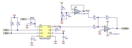
Figure 1-2. LCD Digital VCOM Using the DAC43701
