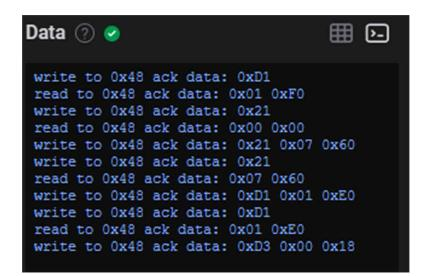
Figure 2-2. I2C Log of the Work Flow
