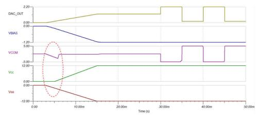
Figure 3-1. Transient Simulation Results When VEE Rises up Earlier
