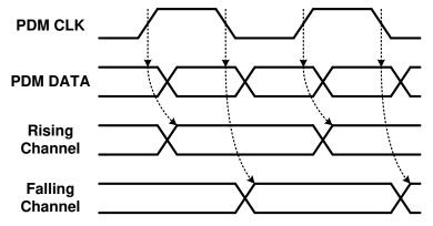
Figure 1-4. PDM Channel Sampling
