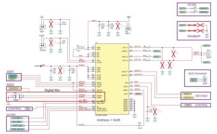
Figure 1-1. PDM Connection Schematic
