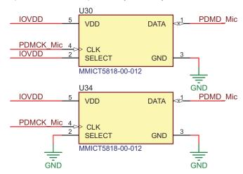
Figure 1-3. PDM Hardware Connections
