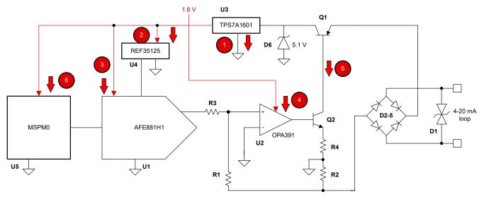
Figure 3. Different Current Components of the Transmitter Circuit
