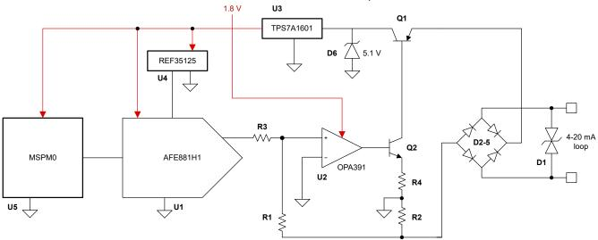
Figure 2. Ultra-Low Power, Low Voltage, 2-Wire 4- to 20-mA Transmitter
