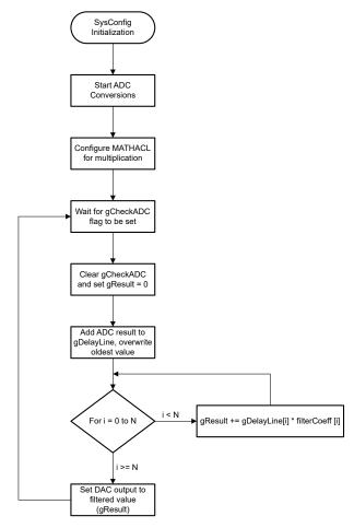
Figure 6-1. Example Software Sequence
