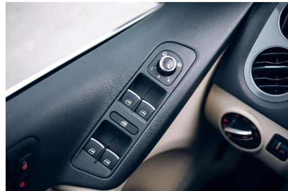
Figure 2. Windows and Mirror Control Switches
