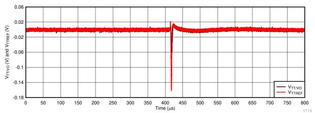
The following are examples of captured waveforms for an SEFI events from run number 109.
