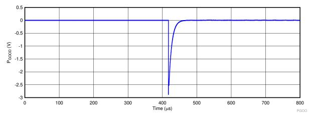
Figure 7-7. The Corresponding  $\rm P_{GOOD}$  Signal Which Flags the Tracking Error Between VTT/V\_O and VTTREF
