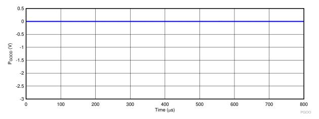
Figure 7-4. P<sub>GOOD</sub> Signal is Not Triggered Since the Set Was Not Big Enough to Cause a Tracking Error
