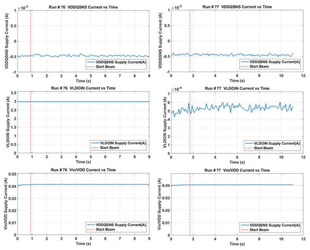
Figure 7-1. SEL Current versus Time (I Versus t) Data in DDR1 Mode for Sourcing (Left) and Sinking 3A (Right)
