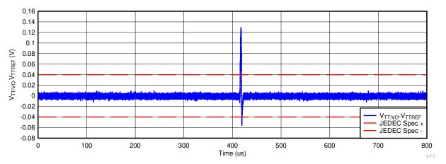
Figure 7-6. The Difference Between VTT/V<sub>O</sub> and VTTREF, Exceeding ±40mV
