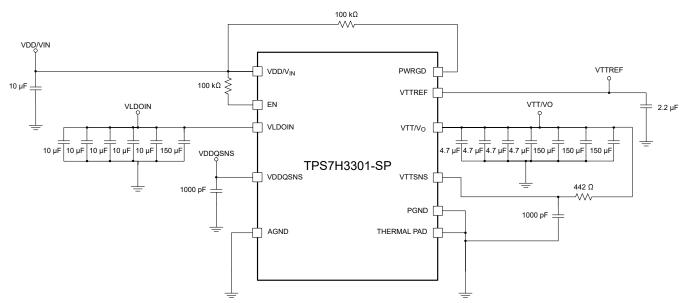
Figure 3-3. Schematic of the Prototype TPS7H3301EVM-CVAL (HREL022) Evaluation Board Used to Perform the SEE Tests on the TPS7H3301-SP Devices
