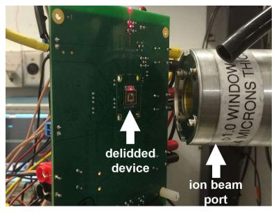
Figure 4-1. Photograph of the TPS7H3301-SP Evaluation Board Mounted in Front of the Heavy Ion Beam Exit Port at the TAMU Accelerator Facility
