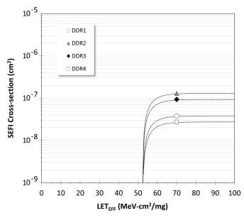
Figure 8-1. SEFI Cross Sections for TPS7H3301-SP as a Function of LET<sub>EFF</sub>
