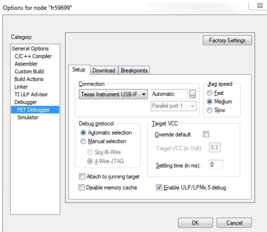
**Figure 2-4. Enable Ultra-Low-Power Debug Mode**
