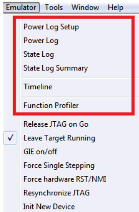
**Figure 3-4. Emulator Pulldown Menu With EnergyTrace++-Related Functions**
