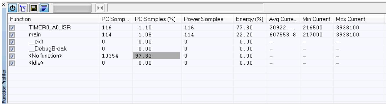
**Figure 3-12. Function Profiler With EnergyTrace++ Data**
