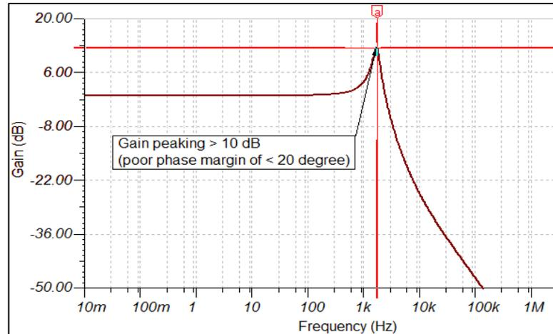
Figure 14: Gain plot – OPA313 with 1 Ohm isolation resistor
