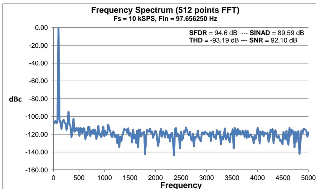
**Figure 1: AC Performance (Measured)**
