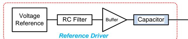
**Figure 6: Capacitor for providing charges (reference drive)**
