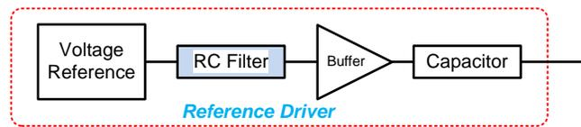
**Figure 5: RC Filter for limiting broadband noise of reference**
