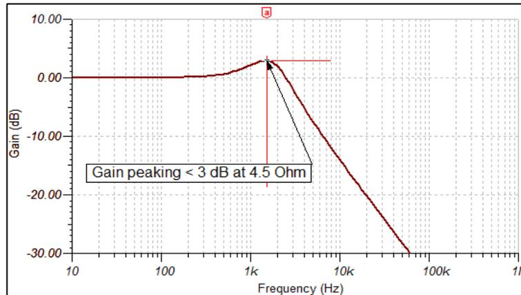
**Figure 16: Gain plot – OPA313 with 4.5 Ohm isolation resistor**
