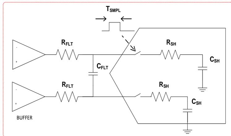
**Figure 9: Input capacitor for attenuating noise**
