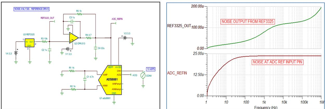
**Figure 30: Noise analysis for reference drive**
