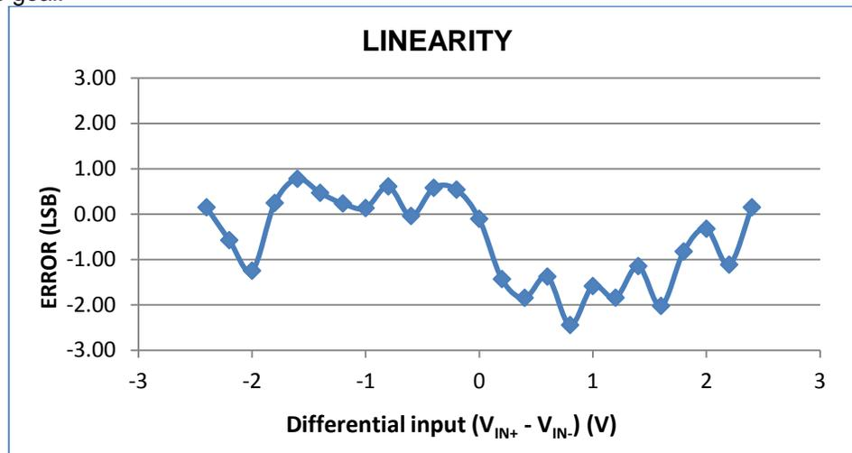
**Figure 35: 25 point linearity check**
