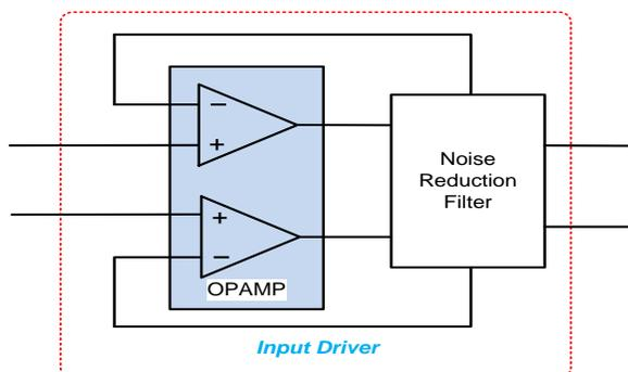
**Figure 11: Buffer driving the input**
