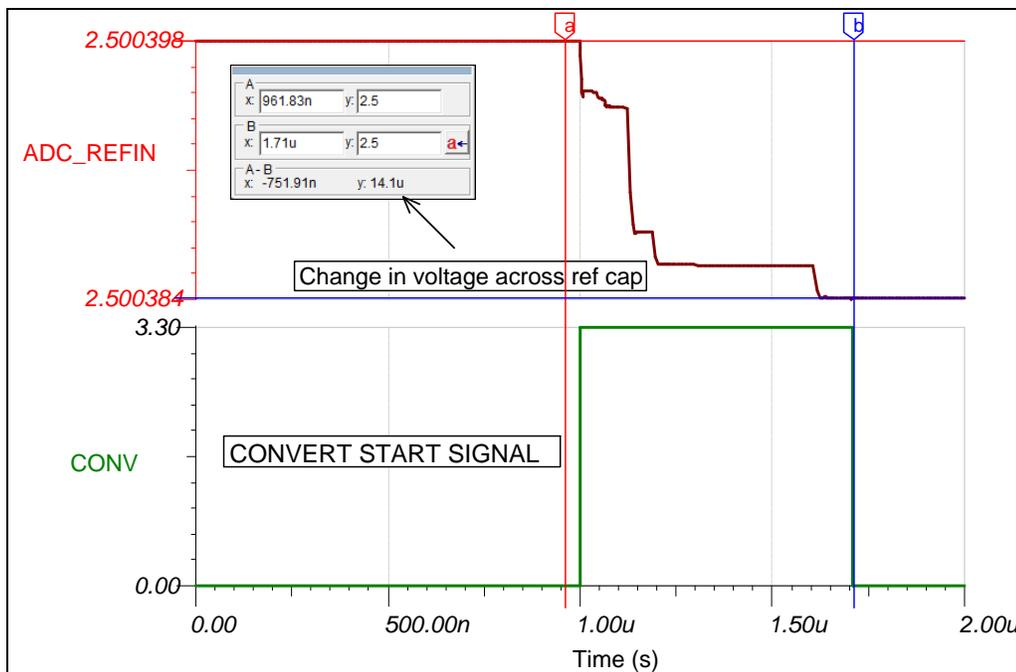
Figure 24: Voltage change across reference capacitor during conversion time
