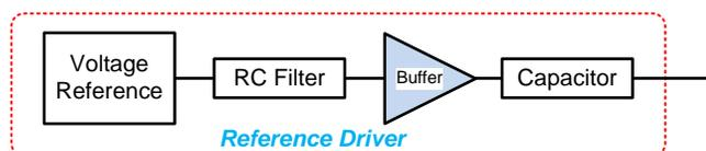
**Figure 7: Buffer for recharging the capacitor**
