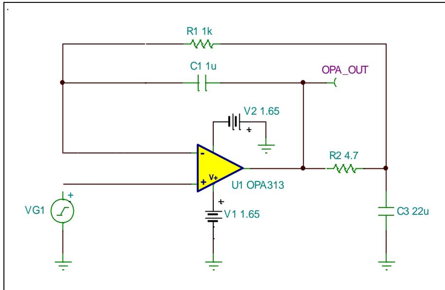
Figure 20: Reference buffer circuit for stability check
