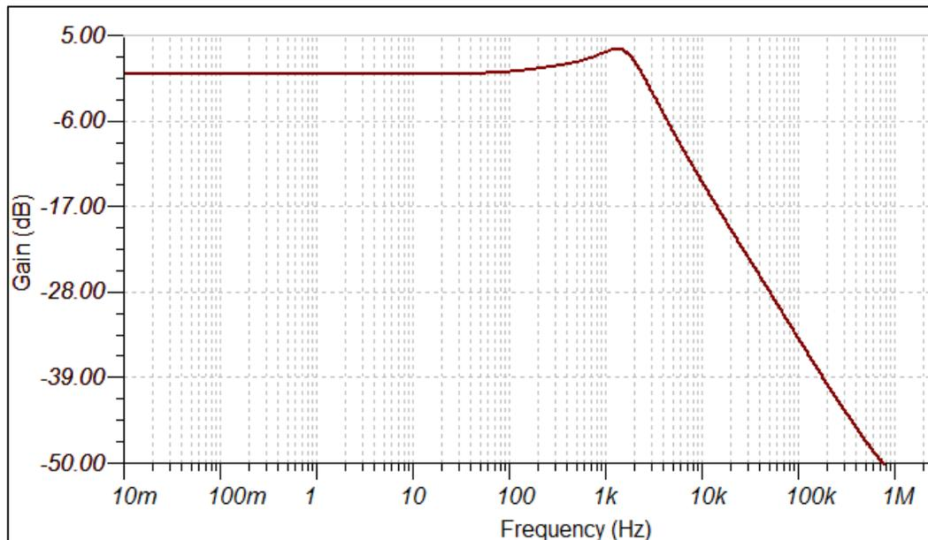
Figure 21: Reference buffer stability check gain plot
