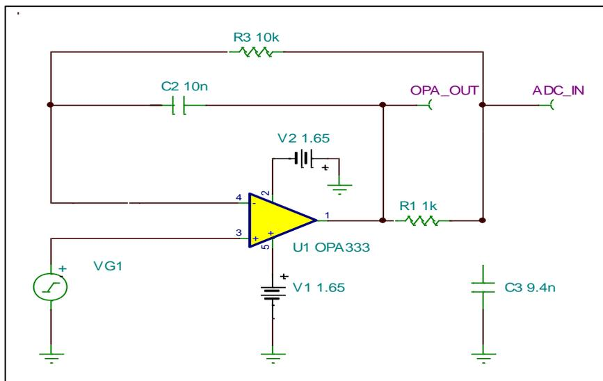
Figure 25: Input buffer circuit for stability check
