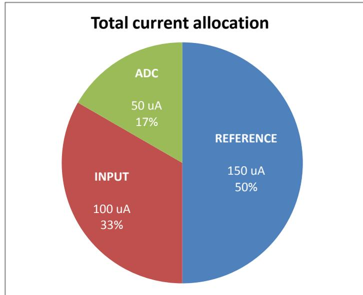
Figure 12: Total current allocation between various blocks
