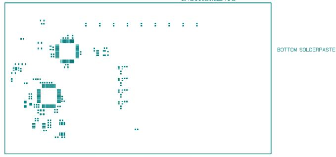
Figure 19. PCM5242EVM Bottom Solderpaste
