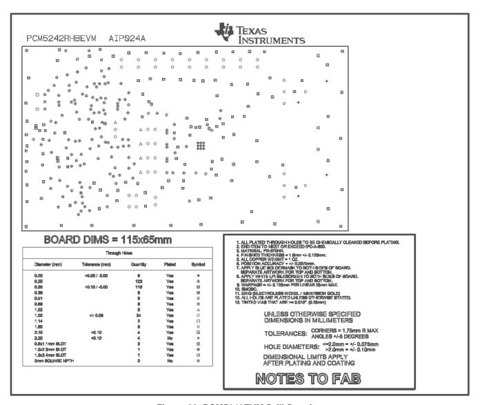
Figure 20. PCM5242EVM Drill Drawing
