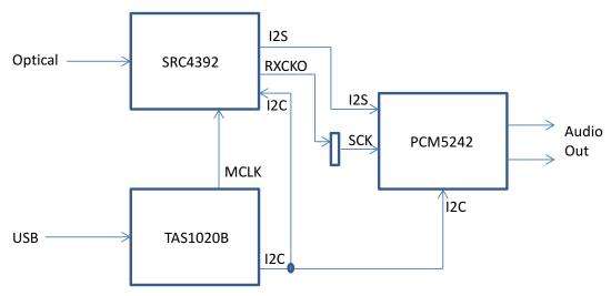
Figure 4. Mode 2 Block Diagram - Optical Audio Input
