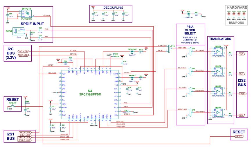
Figure 9. PCM5242EVM Schematic Sample Rate Converter
