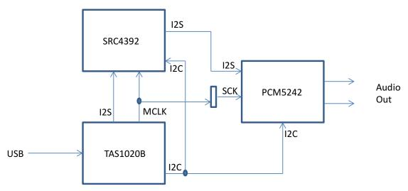
Figure 3. Mode 1 Block Diagram - USB Audio
