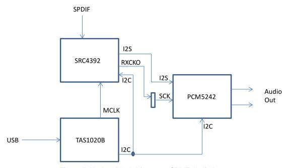
Figure 5. Mode 3 Block Diagram - SPDIF Audio Input
