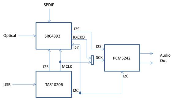
Figure 2. PCM5242EVM Block Diagram
