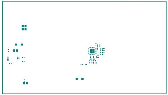
Figure 18. PCM5242EVM Top Solderpaste
