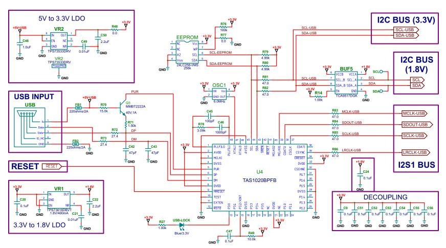
Figure 8. PCM5242EVM Schematic USB to I<sup>2</sup>C/I<sup>2</sup>S Converter
