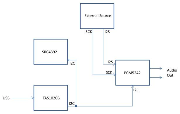
Figure 6. Mode 4 Block Diagram – External Audio Input
