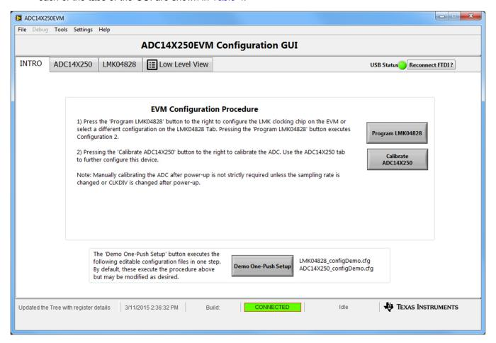
Figure 5. ADC14X250EVM GUI
