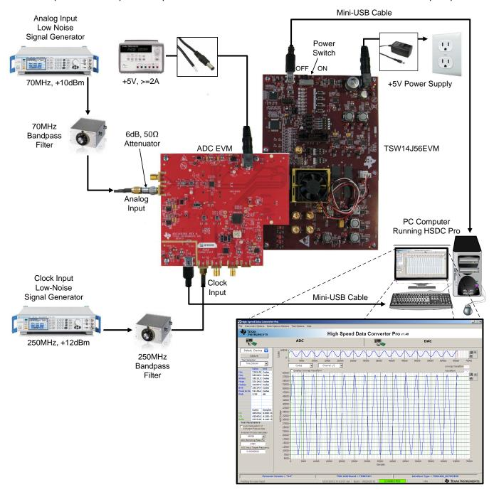
Figure 2. Quick Start Test Setup
