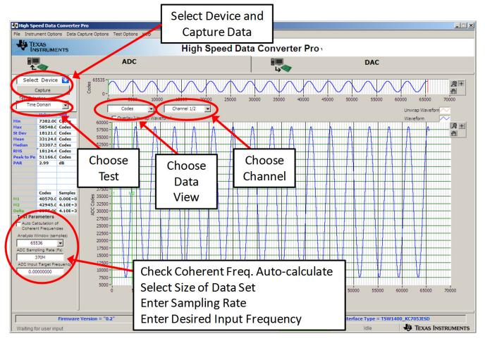
Figure 3. HSDC Pro GUI Main Panel
