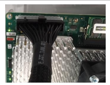
**Figure 6-2. Output Power Cable Connection**
