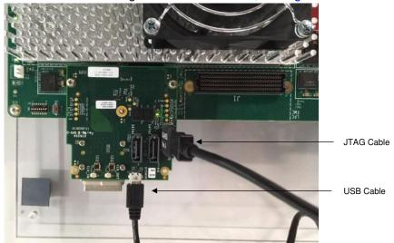
Figure 6-3. JTAG and USB Cable Connections
