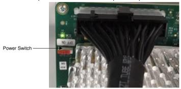
Figure 6-4. Alpha Data Board Power Switch
