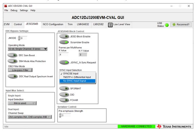
Figure 7-4. Setting ADC to use Software SYNC
