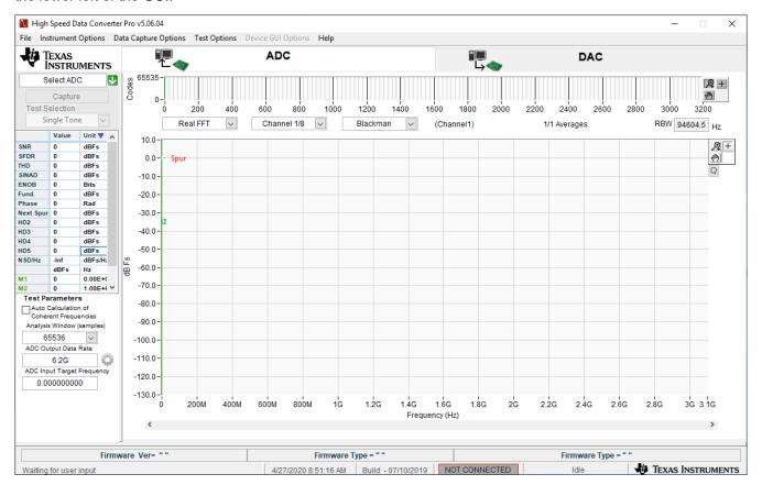
Figure 7-14. Enter ADC Sampling Rate
