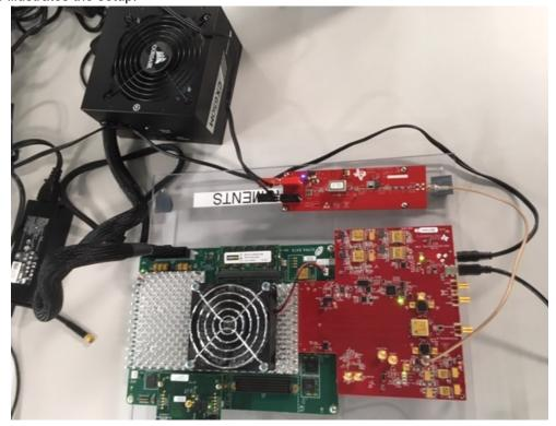
Figure 6-5. Alpha Data Board With ADC12DJ3200 CVAL EVM Setup
