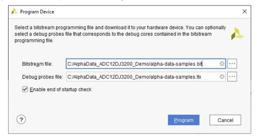
Figure 7-11. Program Device With the bit File
