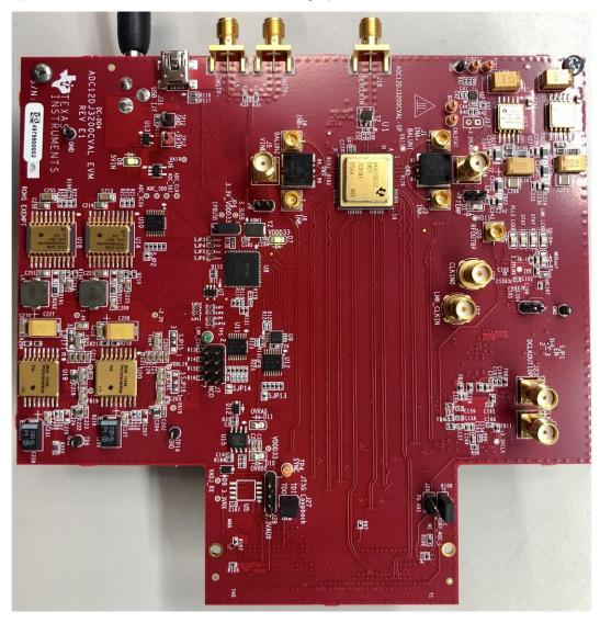
Figure 6-1. ADC12DJ3200EVM Board
