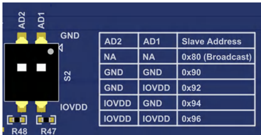
Figure 2-7. DIP Switch S2-S3 for I 2 C Address Selection
