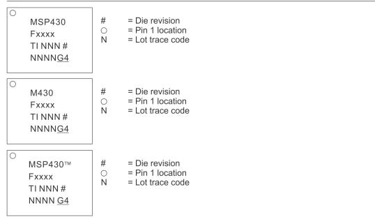
NOTE: Package marking with "TM" applies only to devices released after 2011.
