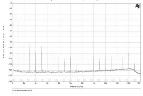
Texas Instruments, Inc. TASS101SE Signal to Noise FFT 10W Output 1kHz Signal Right Channel 06/11/02 14:35:37
