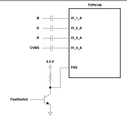
Figure 3. Typical RGB, CVBS, and FSS Connections for SCART
