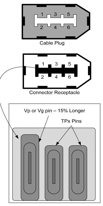
Side View of the Interior of the Connector Receptacle
