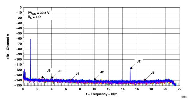
Figure 4–5. FFT, i-kHz Sine Wave at –60 dB
