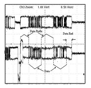
Figure 10. Self-ID Packets for a Six-Port PHY
