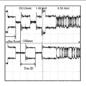
Figure 6. End-of-Bus Reset
