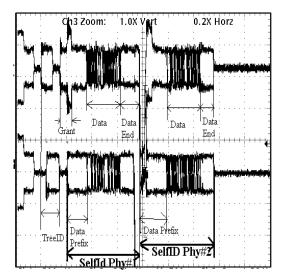
Figure 5. End-of-Bus Reset, Tree-ID, and Self-ID Process
