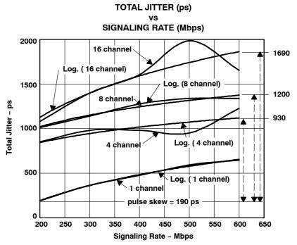
Figure 5. Jitter vs Signaling Rate and Number of Channels
