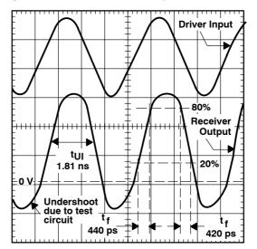
Figure 3. Typical Signals at the Maximum Signaling Rate
