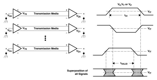
Figure 2. Parallel Operation of Data Interchange Circuits
