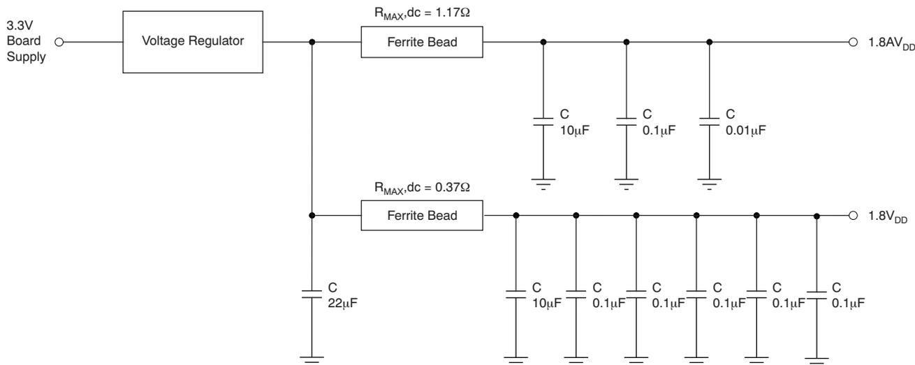
**Figure 16. Power-Supply Decoupling Recommendation**
