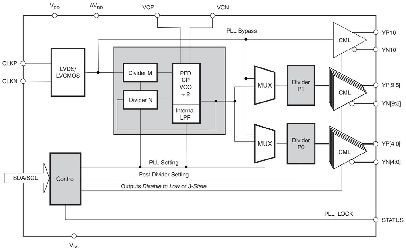
Figure 1. CDCL6010 Block Diagram
