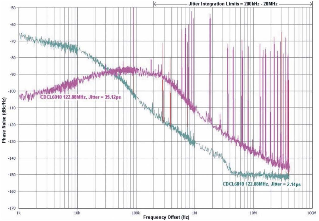
Figure 9. CDCL6010 Input and Output Phase Noise (122.88MHz), Input Jitter = 35.2ps RMS
