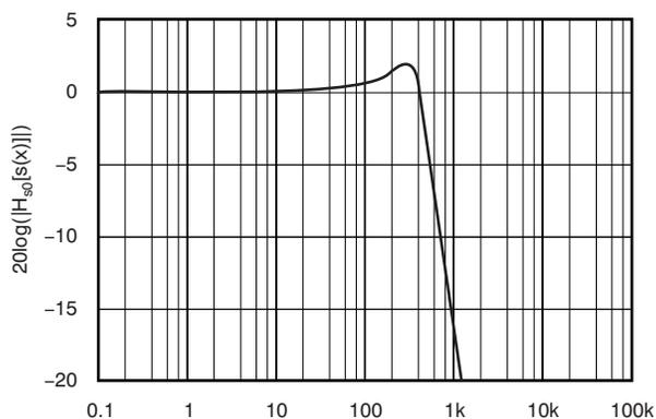
Figure 4. Jitter Peaking Around PLL Bandwidth
