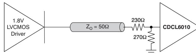
Figure 15. Single-Ended LVCMOS Interface from CDCE706 to CDCL6010
