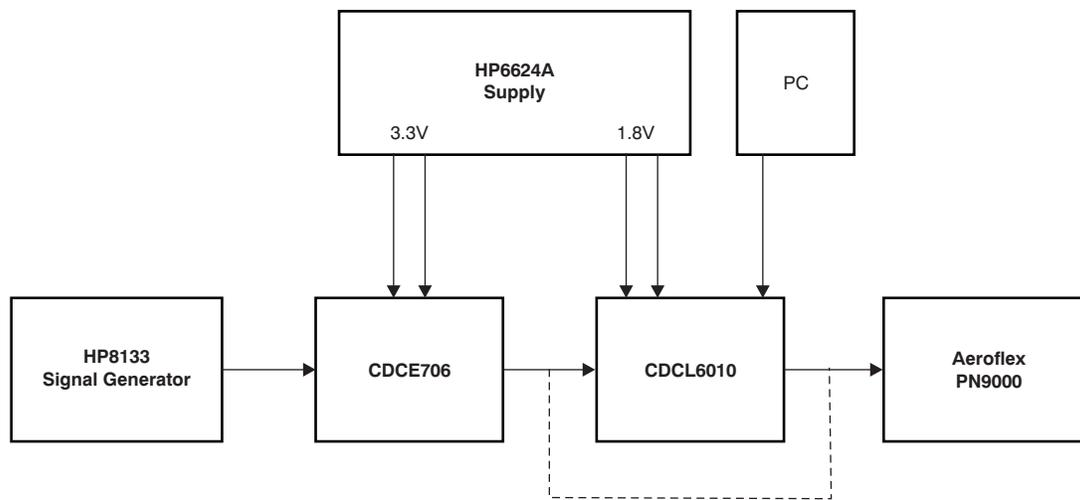
**Figure 6. CDCL6010 Jitter Attenuation Test Setup**
