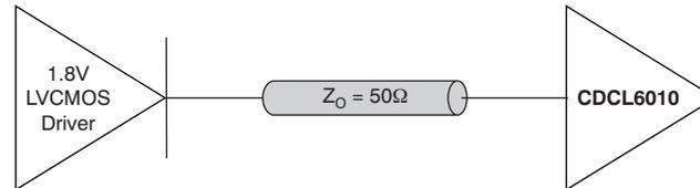
Figure 14. 1.8V Single-Ended LVCMOS Interface to CDCL6010
