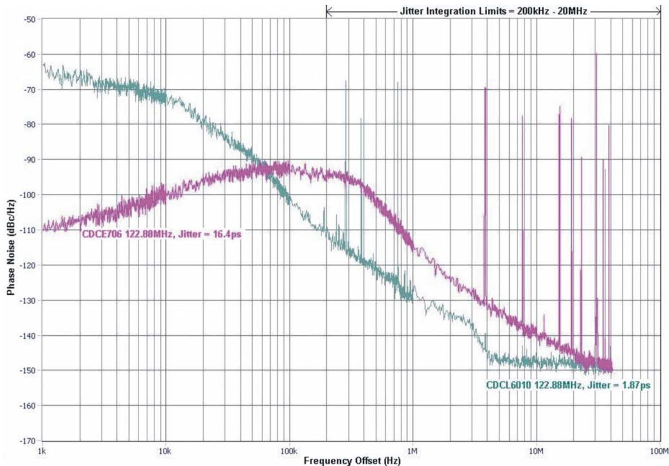
Figure 8. CDCL6010 Input and Output Phase Noise (122.88MHz), Input Jitter = 16.4ps RMS
