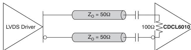
Figure 13. AC-Coupled Input Termination Circuit
