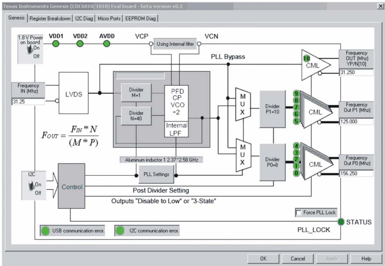
Figure 2. CDCL6010 Programming Settings and Required Input Frequency
