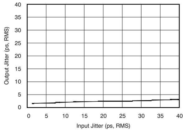
Figure 10. CDCL6010 Jitter Cleaning Capability
