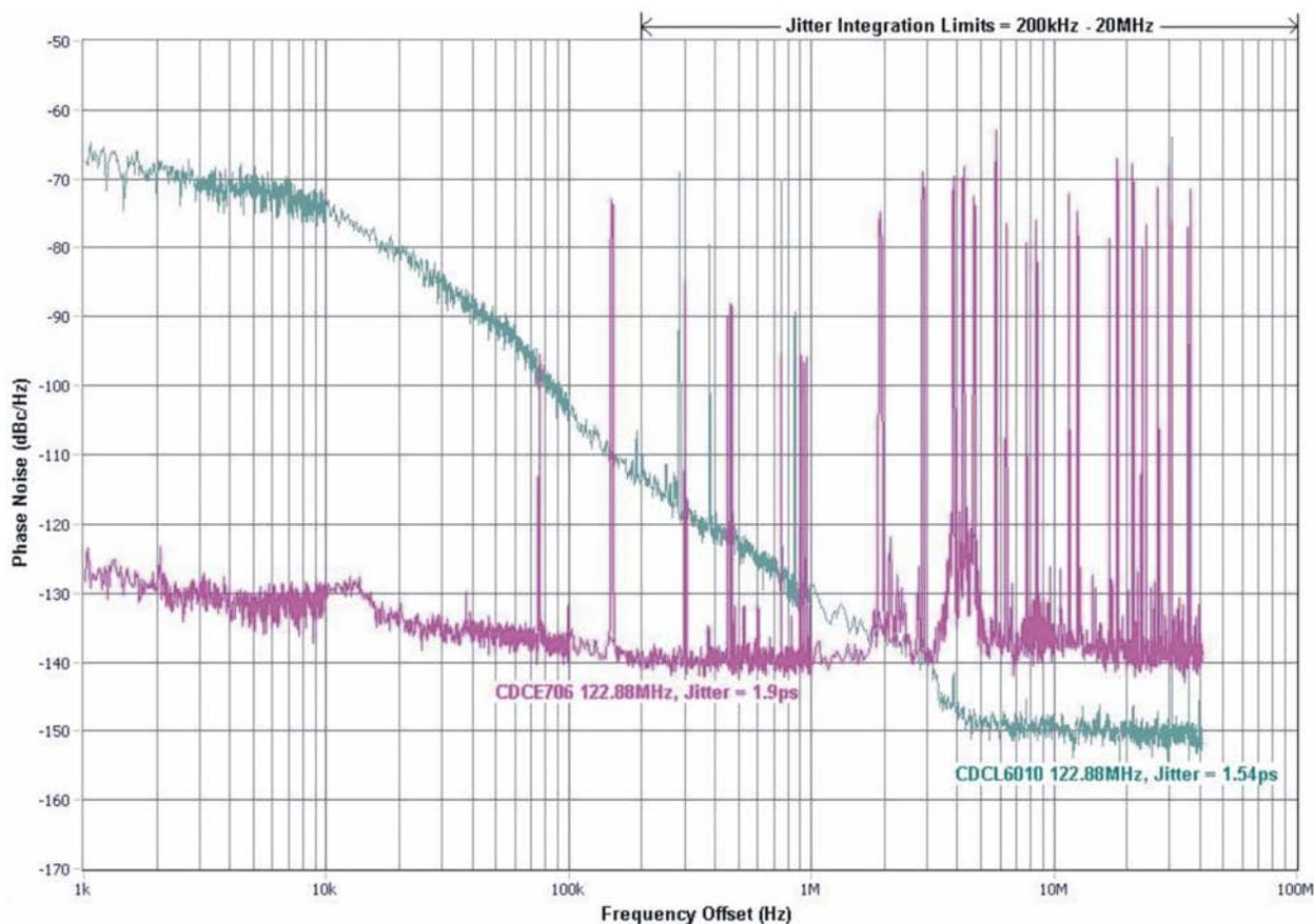
**Figure 7. CDCL6010 Input and Output Phase Noise (122.88MHz), Input Jitter = 1.9ps RMS**
