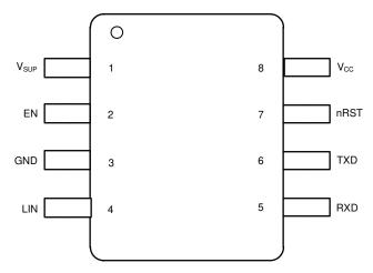
Figure 3-1. Pin Diagram
