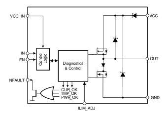
Figure 1. Functional Block Diagram
