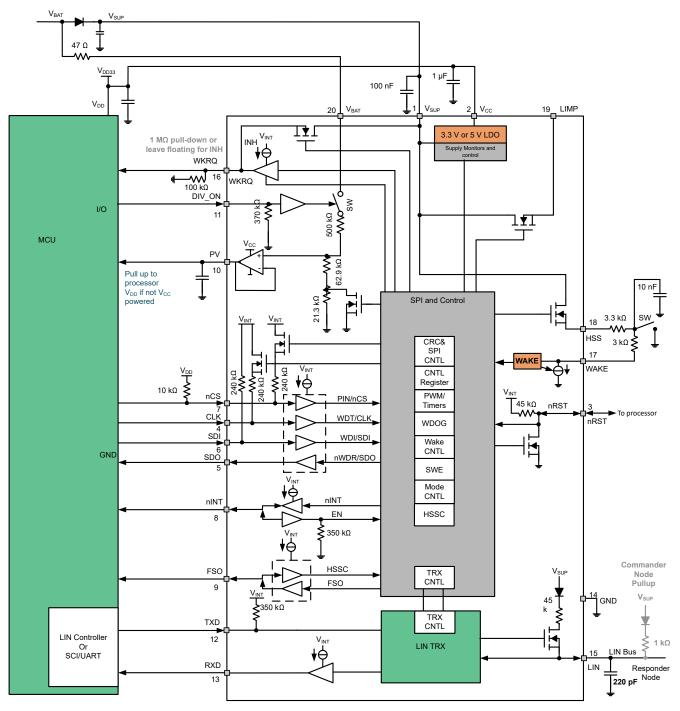
Figure 4-3. Typical Application - SPI Control
