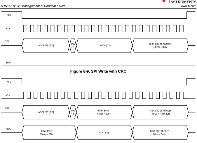
Figure 6-10. SPI Read with CRC
