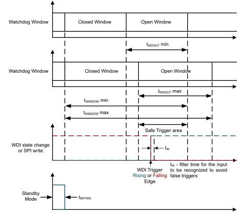
Figure 6-6. Watchdog Timing Diagram
