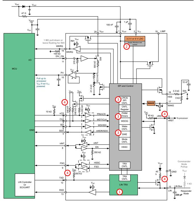
Figure 4-4. Typical Application - SPI Control Potential Failure Points
