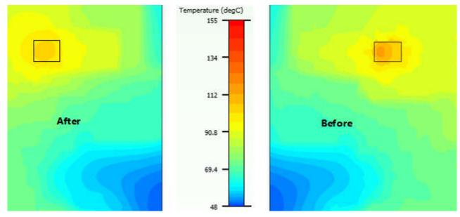
Figure 2-15. Thermal Simulation for MCX831X Layout
