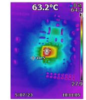
Figure 2-6. MCF8315 Thermal Image in Test 2 Configuration
