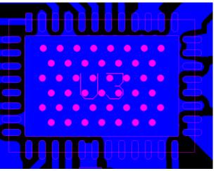
Figure 2-12. MCF831X PCB With More Vias
