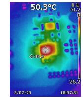
Figure 2-10. MCF8316 Thermal Image in Test 2 Configuration
