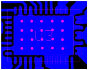
Figure 2-11. MCF831X PCB With Few Vias
