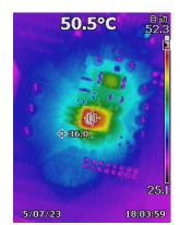
Figure 2-4. MCF8315 Thermal Image in Test 1 Configuration
