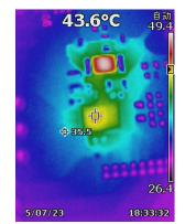
Figure 2-8. MCF8316 Thermal Imagein in test 1 configuration
