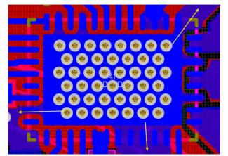
Figure 2-13. MCF831X Heat Dissipation Path (Bottom Layer)
