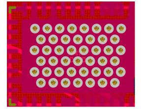
Figure 2-14. MCF831X Heat Dissipation Path (Top Layer)
