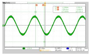
Figure 2-7. MCF8316 Current Waveform in Test 1 Configuration
