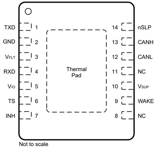
Figure 6-1. DMT Package, 14 Pin (VSON), Top View
