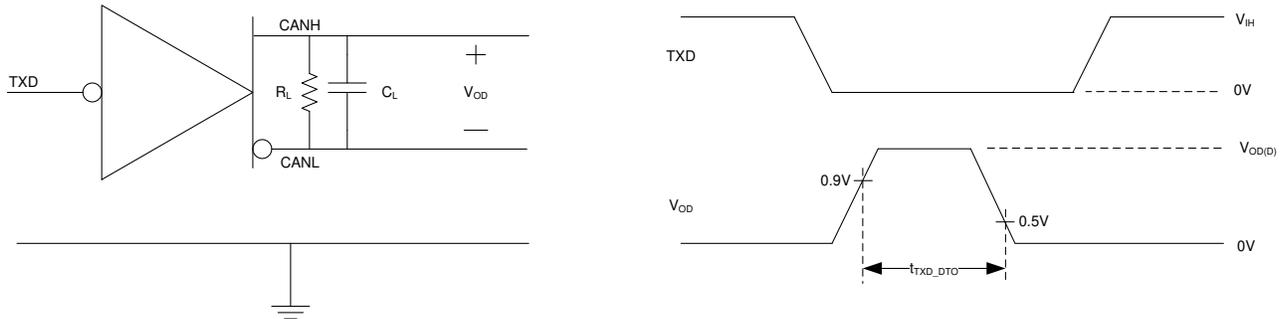
**Figure 8-5. TXD Dominant Timeout Test Circuit and Measurement**
