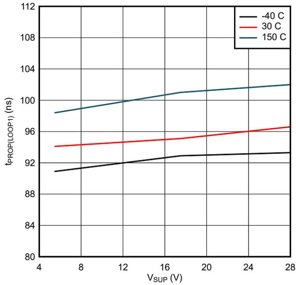
**Figure 7-1.  $t_{PROP(LOOP1)}$  over  $V_{SUP}$**
