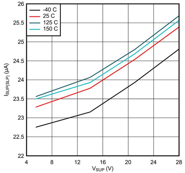
**Figure 7-2.  $I_{SUP}$  over  $V_{SUP}$  Sleep Mode**
