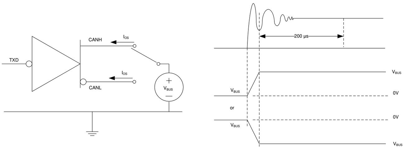
**Figure 8-6. Driver Short-Circuit Current Test and Measurement**
