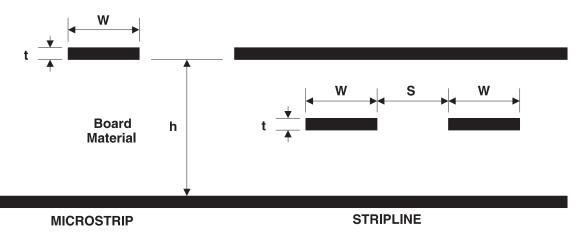
Figure 26. Trace Configurations in Printed-Circuit Boards
