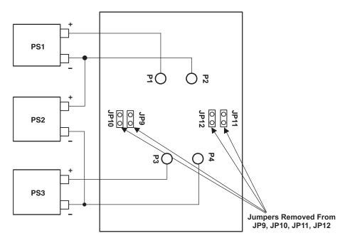
Figure 8. EVM Configuration for Including a Ground Potential Difference Voltage Between Nodes
