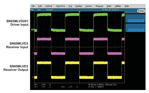
Figure 18. Two-Node Multidrop Typical Eye Pattern at 8 kHz With High-Impedance Output Termination
