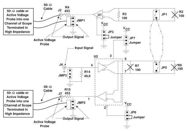
Figure 11. Two-Node Multidrop Transmission
