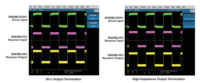
Figure 12. Point-to-Point Simplex Typical Eye Patterns at 8 kHz
