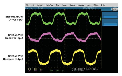
Figure 17. Parallel Terminated Point-to-Point Parallel Simplex Typical Eye Pattern at 125 MHz with High-Impedance Output Termination
