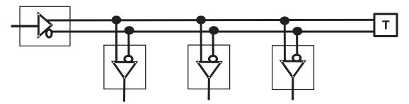
Figure 5. Multidrop or Distributed Simplex Circuit
