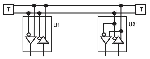
Figure 7. Two-Node Multipoint Circuit
