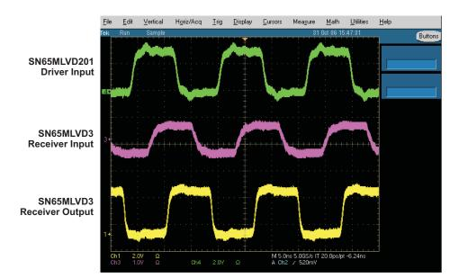
Figure 16. Parallel Terminated Point-to-Point Parallel Simplex Typical Eye Pattern at 61.44 MHz with High-Impedance Output Termination
