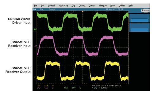
Figure 13. Point-to-Point Simplex Typical Eye Patterns at 61.44 MHz With High-Impedance Output Termination
