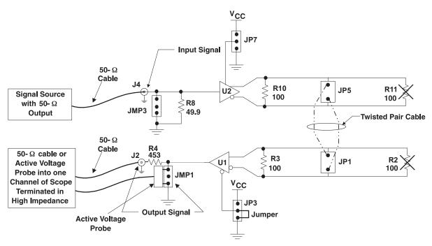
Figure 10. Point-to-Point Parallel Terminated Simplex Transmission
