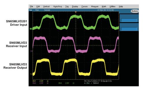
Figure 20. Two-Node Multidrop Typical Eye Pattern at 125 MHz With High-Impedance Output Termination
