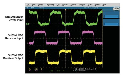
Figure 19. Two-Node Multidrop Typical Eye Pattern at 61.44 MHz With High-Impedance Output Termination
