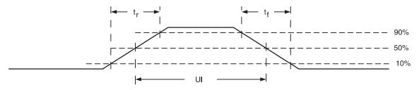
Figure 1. M-LVDS Unit Interval Definition
