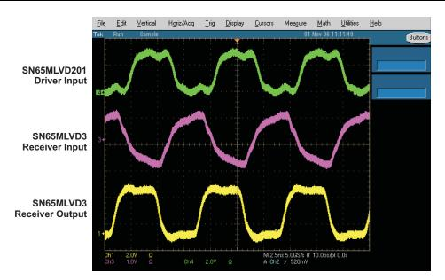
Figure 14. Point-to-Point Simplex Typical Eye Patterns at 125 MHz With High-Impedance Output Termination
