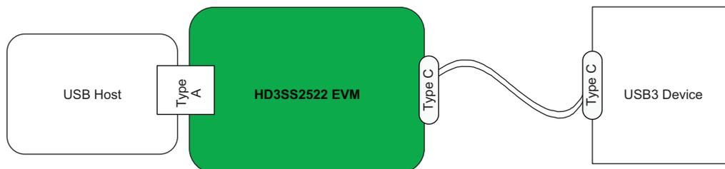
1. Plug the EVM into a USB host with a Type A receptacle via J2
