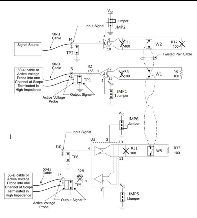
Figure 11. Two-Node Multipoint Transmission
