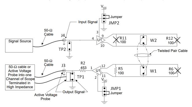
Figure 9. Point-to-Point Simplex Transmission
