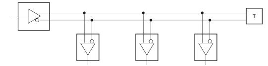
Figure 5. Multidrop or Distributed Simplex Circuit
