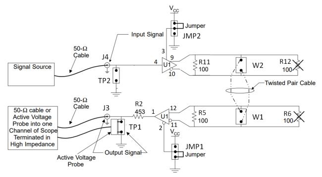
Figure 10. Point-to-Point Parallel Terminated Simplex Transmission
