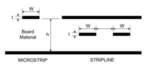
Figure 16. Trace Configurations in Printed-Circuit Boards
