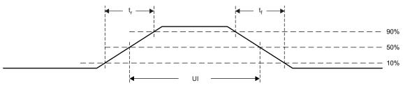
Figure 1. M-LVDS Unit Interval Definition
