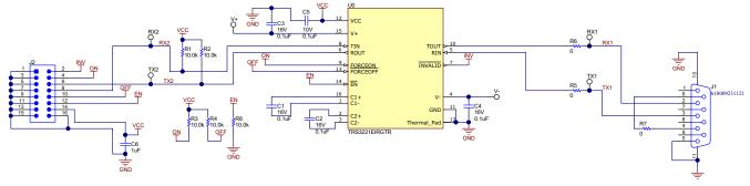
Figure 3-1. TRS3221RGTEVM Schematic
