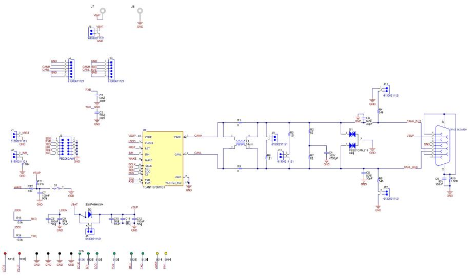
Figure 4-1. TCAN1167EVM CAN Schematic
